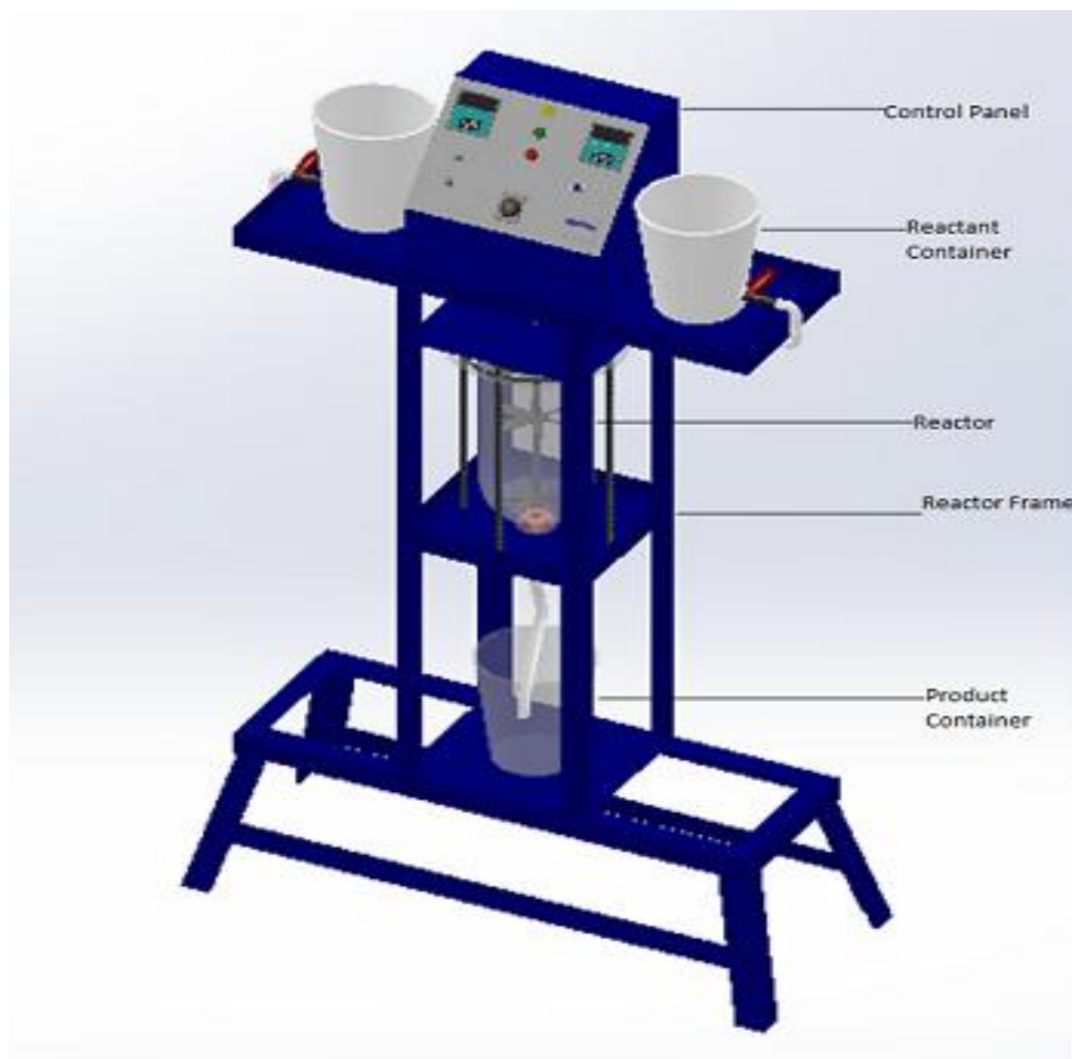
Figure 1 A labelled 3 Dimensional solidworks drawing of the reactor
